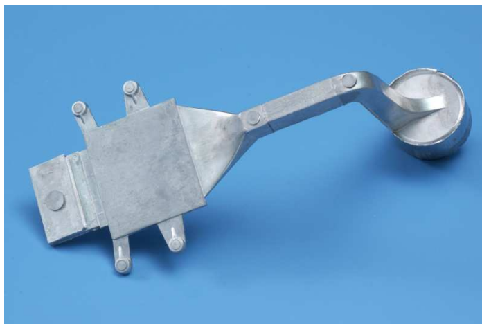
Figure 1. The plate casting showing the complete runner system, overflows, and ejection points.
